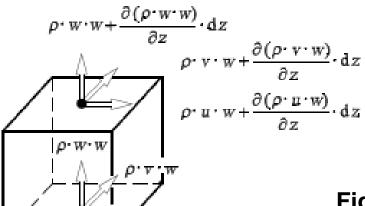
**Figure:** Momentum fluxes entering and exiting the volume element dV
