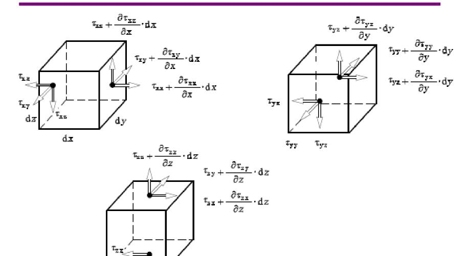
**Figure:** Normal stresses and shear stresses at the volume element dV
