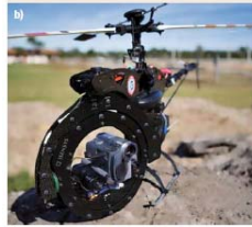
Figure.. Man-packable UAVs used to search portions of Mississippi during the hurricane Katrina response: an ISENSYS IP3 rotary-wing UAV (courtesy of CRASAR)
