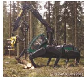
Figure .. Walking forest harvester prototype by Plustech Ltd., today part of John Deere
