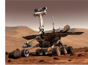
Figure .. The Mars exploration rovers, spirit and opportunity, with a manipulator arm in front
