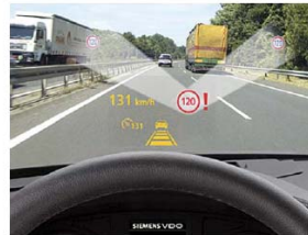
Fig. 51.7 Road sign detection for speed warning application.
