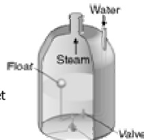
FIGURE 1.2 Water level float regulator,
