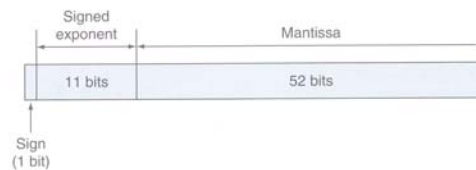
Figure: The manner in which a floating point number is stored in IEEE double precision format
